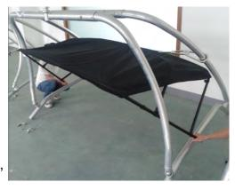
Now you shall put aside the bimini top for a moment and mount the four bimini rings in according to the marks ,
